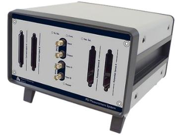
The Quasi-DC Potential Drop Monitoring System utilises very low frequency (0.3-30Hz) measurements, combining the benefits of both DC and AC Potential Drop measurements (DCPD and ACPD respectively).
